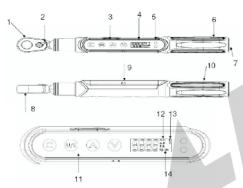
1 Reversible ratch head 2 Direction lever 3 Communication port 4 LCD readout 5 LED Indicator 6 Anti-slip Handle 7 Battery Cover
