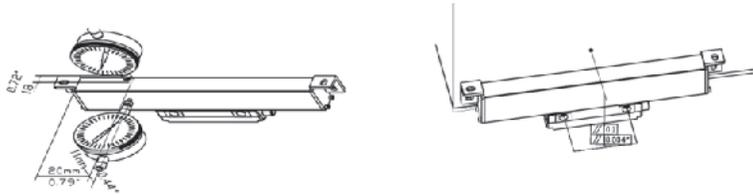
9 The crooked radius of the signal cable should be more than 60mm.
