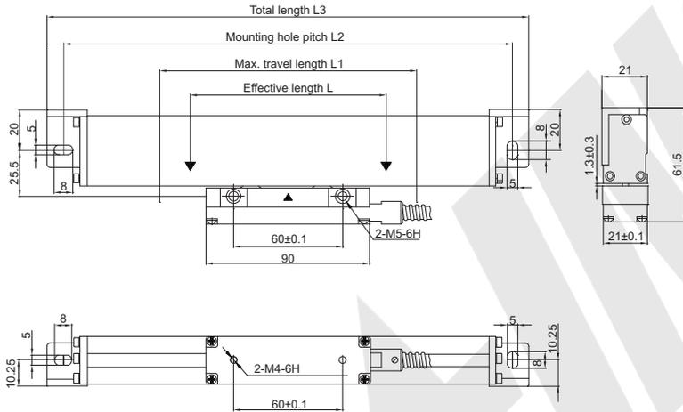
b Installation figure of ISL-B5 series linear scale.
